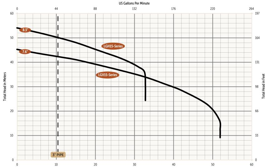
Pumps must operate within the proper range shown on the performance of the performance of the end user to ensure this requirement is met. Pumps operating outside the recommended range are prone to damage, excessive vibration, cavitation, poor efficiency, and may exceed nameplate amperage.
